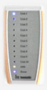
The Handheld Alert Device (HAD) can monitor up to 10 Sensor Devices (MSD).
