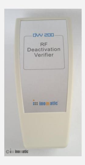
The Deactivation Verifier DVV-200 allows easy checking of the deactivation height of the deactivator. It works on a frequency of 8.2MHz.
