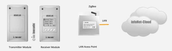
The LAN Access Point allow the operation of up to **100 Visitor Counter Receiver modules**. The communication between the RX Visitor counter and the LAN Access Point is via ZigBee. The ZigBee protocol provides for a stable and safe communication between the Visitor counter and the LAN Access point
